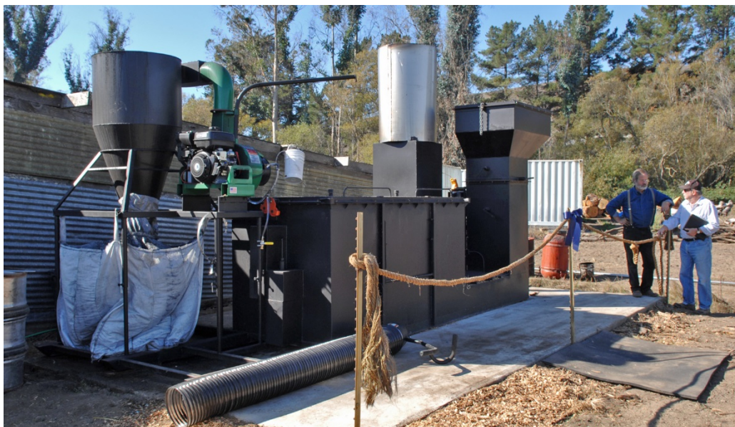
SEC's Adam Retort Biochar Production Unit
